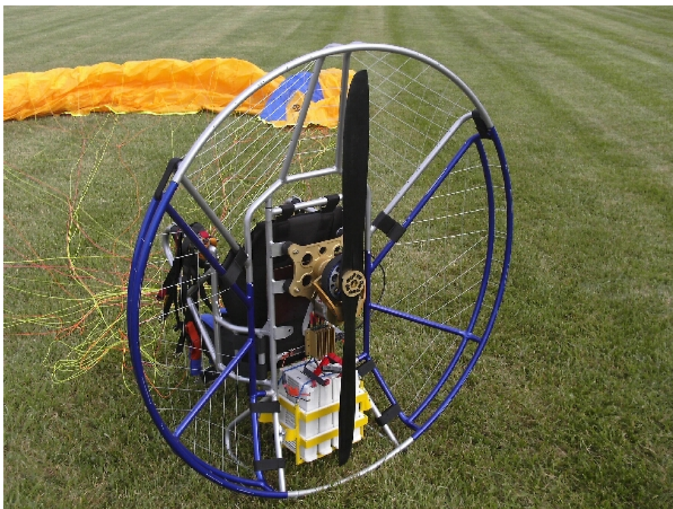
Worlds First Electric Paraglider powered by Lipo Batteries.
